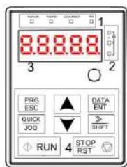
Figure 4-2 Keypad diagram for inverters \geq 4\text{kW}
